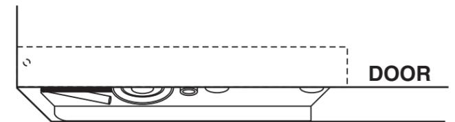
5. Install Door. Turn closing speed valves shut (clockwise).
