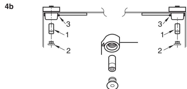
**CAUTION:** Closer is shipped with Closing Speed valve down. DO NOT FORCE VALVE DOWN.
