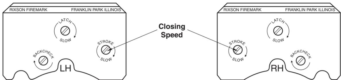
Closing speeds can be adjusted to suit local conditions and requirements. Label on closer face designates the purpose of each adjustment screw.
