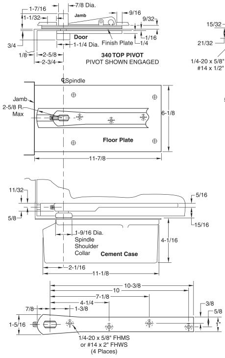
Conversion from inches to metric: inch x 25.4. Suitable reinforcing by others. Rixson designed threshold available on request.
