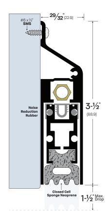
This product may be used to restore lost fire ratings due to excessive gaps at the bottom of the door up to 1-1/2 when installed per NFPA 80.
