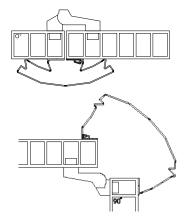
We recommend using tape on metal, aluminium & PVC doors and frames. It is often not possible to fit the narrow strip because of a different hinge type, unless the narrow strip and click strip are cut and fitted above and below the unprotected hinge. We strongly advise against this!
