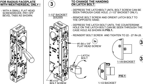
TO CHANGE THE HANDING - YOU WILL ALSO HAVE TO RE-ORIENT THE INTER-CONNECT CAM: - DEPRESS THE LATCHBOLT UNTIL BOLT SCREW CAN BE a) LOOSEN THE #6-32 FLAT HEAD SCREW AT THE BOTTOM OF THE LOCK.
