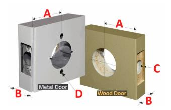
IMPORTANT NOTE FOR WOOD DOORS: Unless known to be factory prepared, all wood doors should have their preparation work carefully checked for dimensional accuracy. All measurements must be within +/- 1/16" (2 mm) of the listed values. If the bore hole or cross-bore hole is drilled out of square the latch may not properly align with the housing. To remedy this, re-drill the problematic hole with the corrected alignment.
