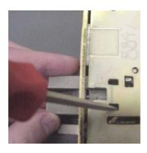
Step 3. Insert screw driver in hole press on Plate while pulling out latch bolt.
