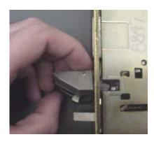
Step 4. Rotate Latchbolt 180<sup>0</sup> to desired handing position.
