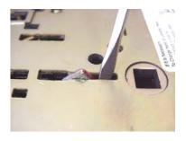
Step 3. Push on edge of Locking Piece between Locking Piece and and Square Spindle Hole.
