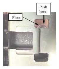
Step 2. Exploded view of Plate where screw driver presses.
