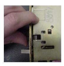
Step 5. Firmly press Latchbolt into case until it stops moving.
