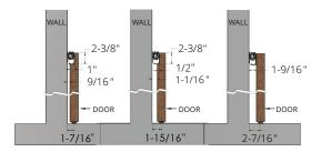
Note: Depth of top route determines clearance between wall and door.
