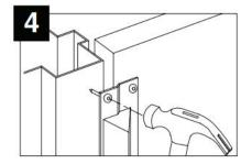
Swing door closed until security pin touches the frame. Mark hole location by hitting head of security pin with hammer.
