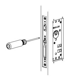
Tighten locking screw to engage notch on cylinder
