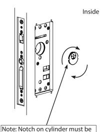
in the 9 o' clock position when fully screwed into lock body.
