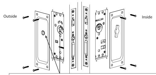
Align Passage/Privacy Button with Thumb-Turn spindle and secure trim plates to door.
