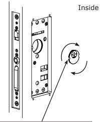
Note: Notch on cylinder must be in the 9 o' clock position when fully screwed into lock body.
