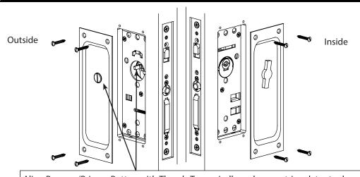
Align Passage/Privacy Button with Thumb-Turn spindle and secure trim plates to door.
