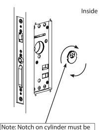
Note: Notch on cylinder must be in the 9 o' clock position when fully screwed into lock body.
