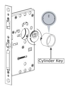
Note: Notches on cylinder must be parallel with the horizontal plane when fully screwed into lock body.
