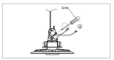
4. Tighten screws to secure mounting bolt hook. (see Figure 4).
