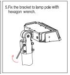
Notice: The maximum diameter of lamp pole is 2.36". lamp adjustable angle is 0-90°.
