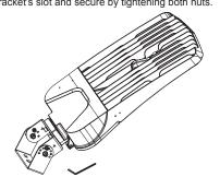
6. With the weight of the luminaire supported so that it does not fall over, secure the base with fixture with two bolts.
