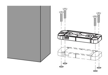
**3**. Use floor plate adjustments to align patch fitting in opening.
