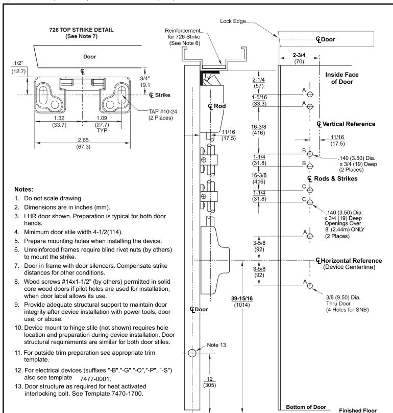
6170-LBR, 6170F90-LBR, 6170-LBR-10, 6170F90-LBR-10 7170W-LBR, 7170WF90-LBR, 7170W-LBR-10, 7170WF90-LBR-10 Surface Vertical Rod Exit Devices
