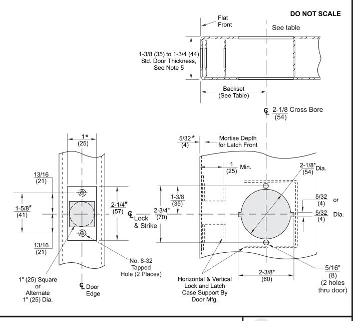
5300LN Series Lever Handle Cylindrical Locks - 1" Wide Flat Front H.M. Door Preparation (See ANSI/BHMA A156.115)
