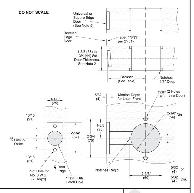
5400LN Series Key-In-Lever Cylindrical Locks - 1-1/8" Wide Front Wood Door Preparation (See ANSI/BHMA A156.115)
