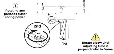
The CA1600 Non Hold Open Closer - Top Jamb Mount has now been installed.
