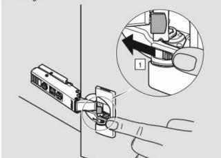
Door must be closed once for the deactivation to be complete. To reactivate, move switch back to original position.
