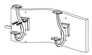
STEP 2: FIX HOOKS WITH TWO WOOD SCREWS AND FINISH WITH COVER CAP
