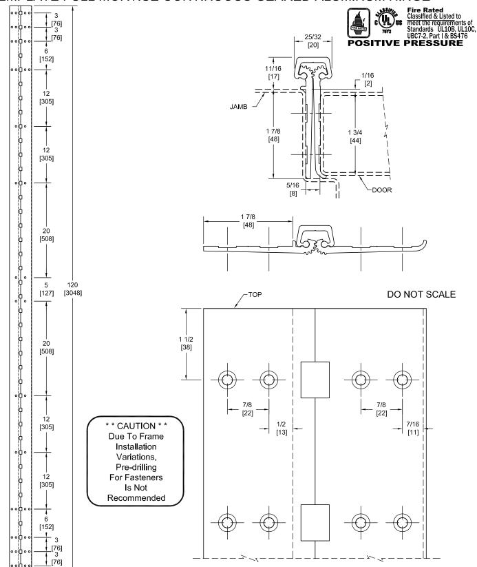
PEMKO Template Full Mortise Continuous Geared Aluminum Hinges CFM120HD/DFM120HD are made to conform to this drawing. PEMKO CFM120HD/DFM120HD hinges can be supplied with Electric Functions - See Electrical Application Section. Machine Screw Size - No. 12-24 x 7/16 FHUC Thread-forming.
