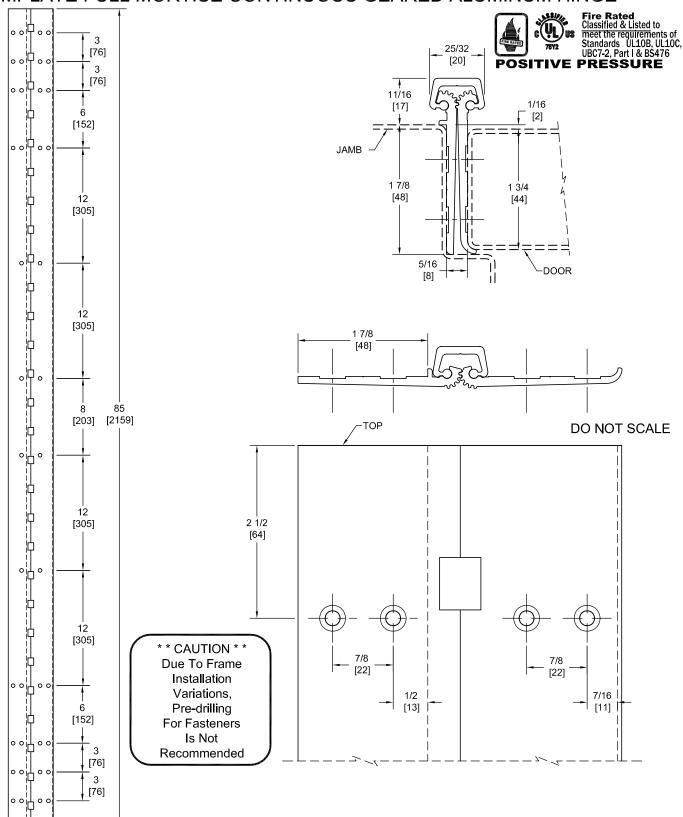
PEMKO Template Full Mortise Continuous Geared Aluminum Hinges CFM85HD/DFM85HD are made to conform to this drawing. PEMKO CFM85HD/DFM85HD hinges can be supplied with Electric Functions - See Electrical Application Section. Machine Screw Size - No. 12-24 x 7/16 FHUC Thread-forming.
