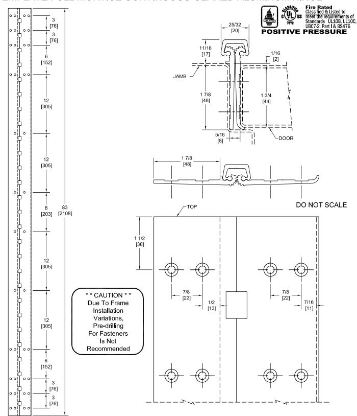
PEMKO Template Full Mortise Continuous Geared Aluminum Hinges CFM83HD/DFM83HD are made to conform to this drawing. PEMKO CFM83HD/DFM83HD hinges can be supplied with Electric Functions - See Electrical Application Section. Machine Screw Size - No. 12-24 x 7/16 FHUC Thread-forming.
