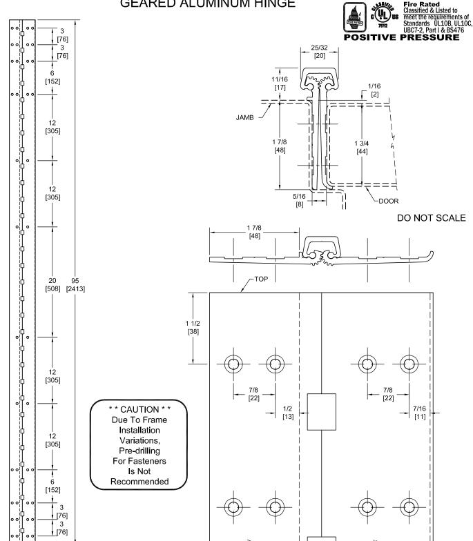
PEMKO Template Full Mortise Continuous Geared Aluminum Hinges CFM95HD/DFM95HD are made to conform to this drawing. PEMKO CFM95HD/DFM95HD hinges can be supplied with Electric Functions - See Electrical Application Section. Machine Screw Size - No. 12-24 x 7/16 FHUC Thread-forming.
