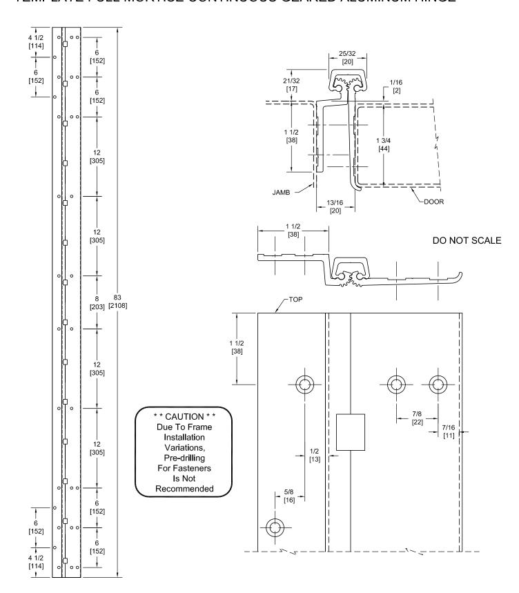
PEMKO Template Full Mortise Continuous Geared Aluminum Hinges CFM83SF/DFM83SF are made to conform to this drawing. Machine Screw Size - No. 12-24  $\times$  7/16 FHUC Thread-forming.
