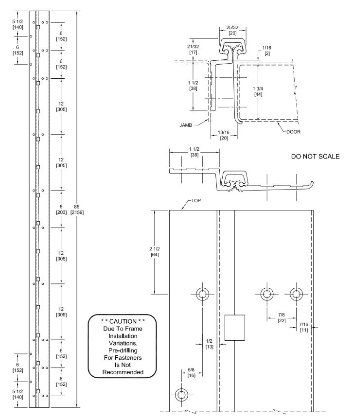
PEMKO Template Full Mortise Continuous Geared Aluminum Hinges CFM85SF/DFM85SF are made to conform to this drawing. Machine Screw Size - No.  $12-24 \times 7/16$  FHUC Thread-forming.
