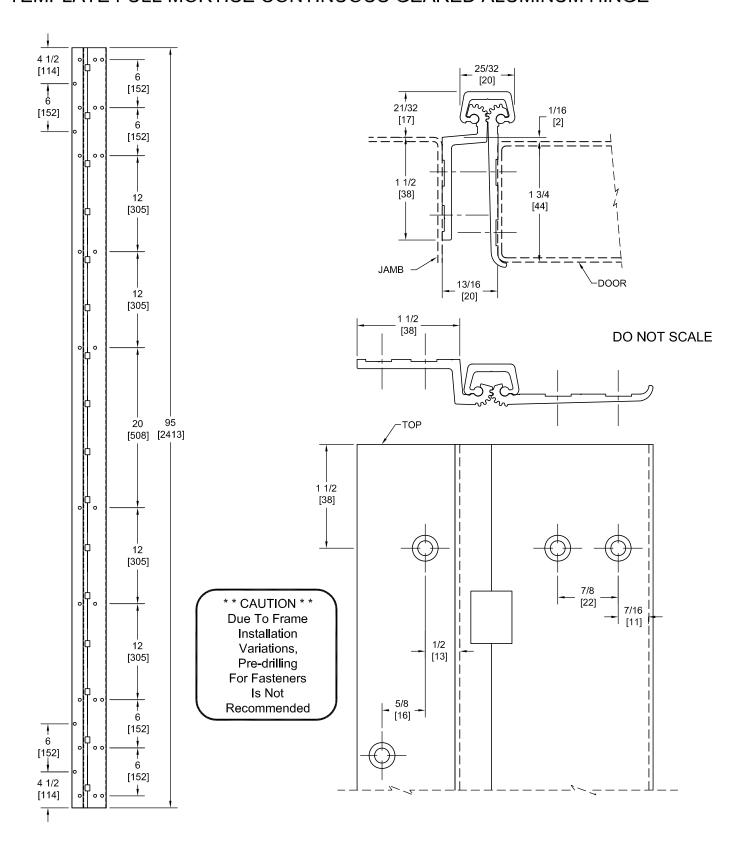
PEMKO Template Full Mortise Continuous Geared Aluminum Hinges CFM95SF/DFM95SF are made to conform to this drawing. Machine Screw Size - No. 12-24  $\times$  7/16 FHUC Thread-forming.
