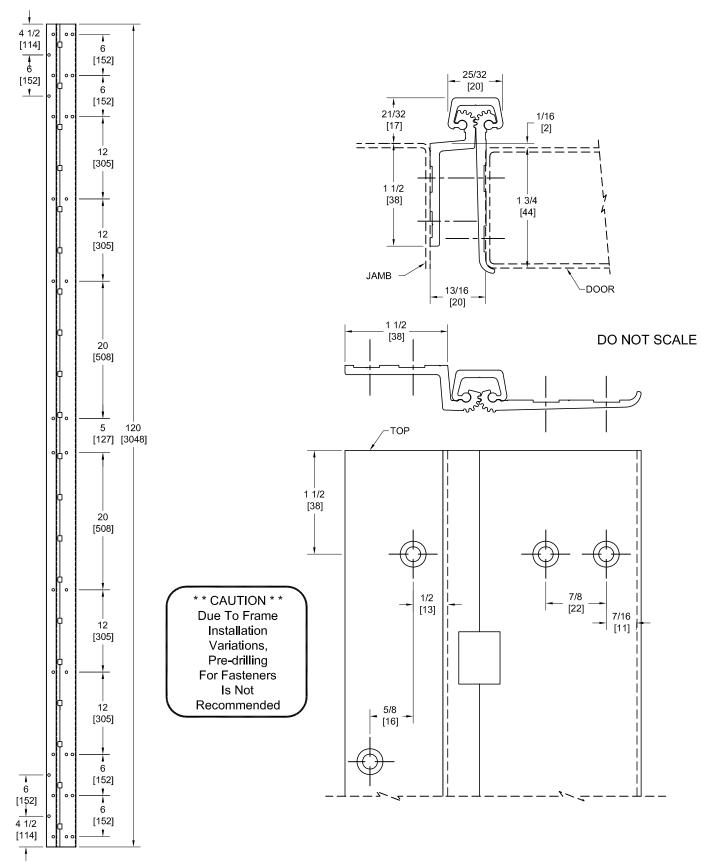
PEMKO Template Full Mortise Continuous Geared Aluminum Hinges CFM120SF/DFM120SF are made to conform to this drawing. Machine Screw Size - No. 12-24  $\times$  7/16 FHUC Thread-forming.
