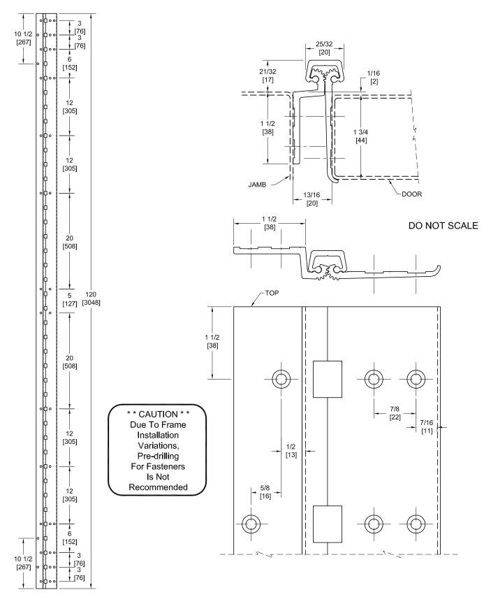
PEMKO Template Full Mortise Continuous Geared Aluminum Hinges CFM120SFHD/DFM120SFHD are made to conform to this drawing. Machine Screw Size - No. 12-24 x 7/16 FHUC Thread-forming.
