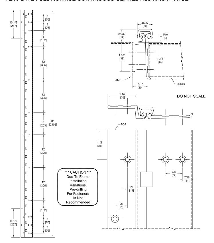
PEMKO Template Full Mortise Continuous Geared Aluminum Hinges CFM83SFHD/DFM83SFHD are made to conform to this drawing. Machine Screw Size - No. 12-24 x 7/16 FHUC Thread-forming.
