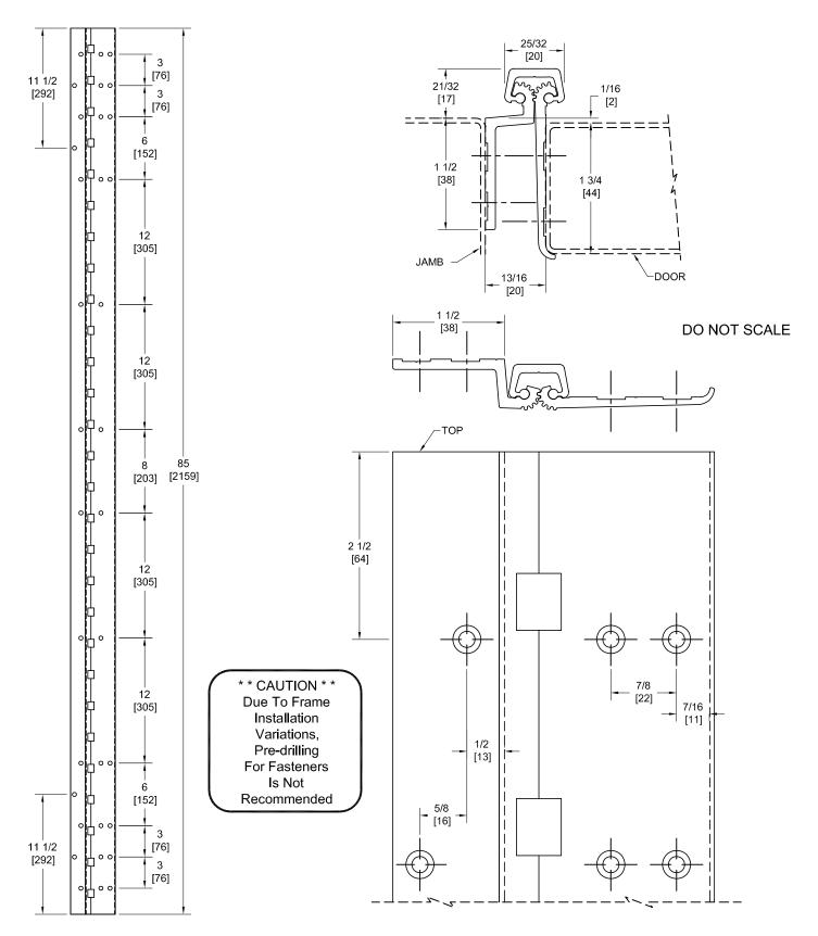
PEMKO Template Full Mortise Continuous Geared Aluminum Hinges CFM85SFHD/DFM85SFHD are made to conform to this drawing. Machine Screw Size - No. 12-24 x 7/16 FHUC Thread-forming.
