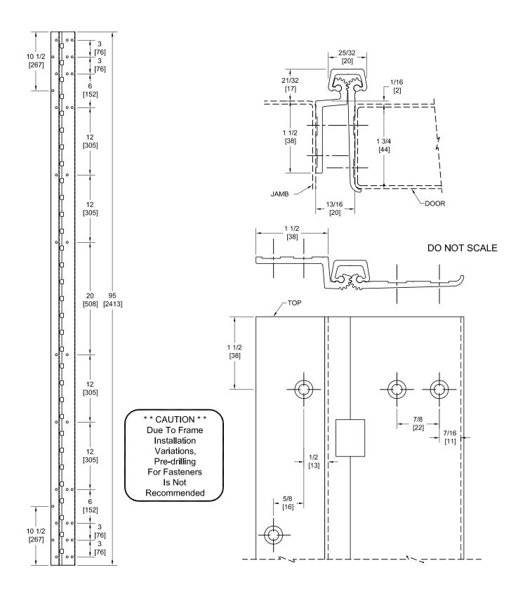
PEMKO Template Full Mortise Continuous Geared Aluminum Hinges CFM95SFHD/DFM95SFHD are made to conform to this drawing. Machine Screw Size - No. 12-24 x 7/16 FHUC Thread-forming.
