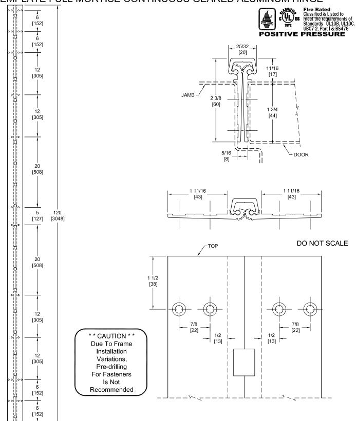
PEMKO Template Full Mortise Continuous Geared Aluminum Hinges CFM120SLF/DFM120SLF are made to conform to this drawing. PEMKO CFM120SLF/DFM120SLF hinges can be supplied with Electric Functions - See Electrical Application Section. Machine Screw Size - No. 12-24 x 7/16 FHUC Thread-forming.
