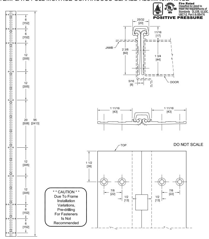
PEMKO Template Full Mortise Continuous Geared Aluminum Hinges CFM95SLF/DFM95SLF are made to conform to this drawing. PEMKO CFM95SLF/DFM95SLF hinges can be supplied with Electric Functions - See Electrical Application Section. Machine Screw Size - No. 12-24 x 7/16 FHUC Thread-forming.
