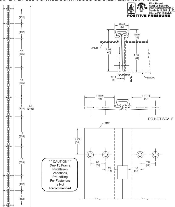
PEMKO Template Full Mortise Continuous Geared Aluminum Hinges CFM83SLF/DFM83SLF are made to conform to this drawing. PEMKO CFM83SLF/DFM83SLF hinges can be supplied with Electric Functions - See Electrical Application Section. Machine Screw Size - No. 12-24 x 7/16 FHUC Thread-forming.
