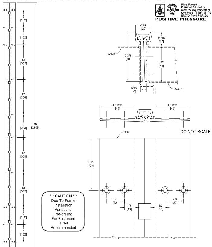
PEMKO Template Full Mortise Continuous Geared Aluminum Hinges CFM85SLF/DFM85SLF are made to conform to this drawing. PEMKO CFM85SLF/DFM85SLF hinges can be supplied with Electric Functions - See Electrical Application Section. Machine Screw Size - No. 12-24 x 7/16 FHUC Thread-forming.
