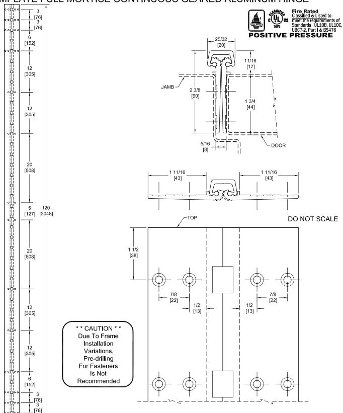
PEMKO Template Full Mortise Continuous Geared Aluminum Hinges CFM120SLF-HD/DFM120SLF-HD are made to conform to this drawing. PEMKO CFM120SLF-HD/DFM120SLF-HD hinges can be supplied with Electric Functions - See Electrical Application Section. Machine Screw Size - No. 12-24 x 7/16 FHUC Thread-forming.
