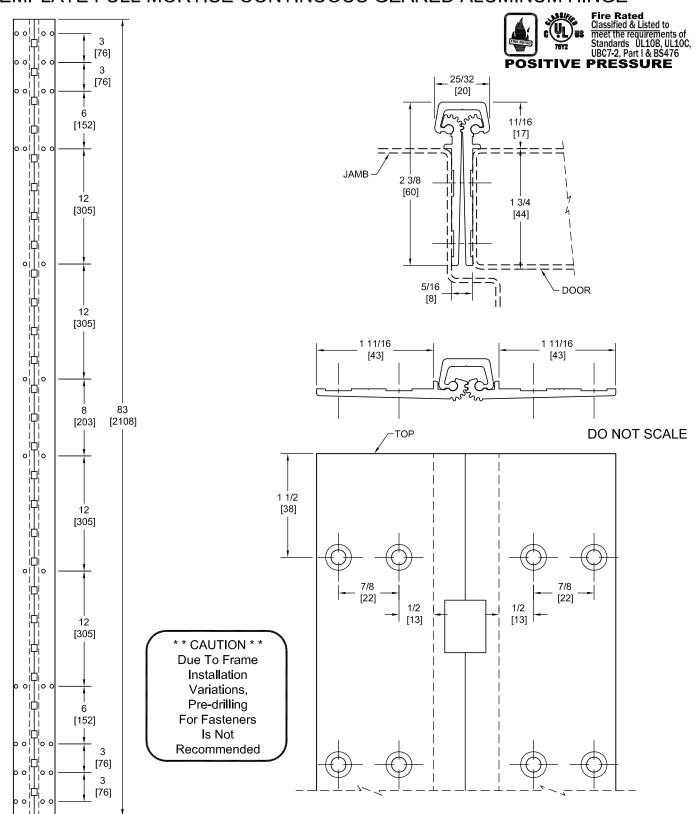
PEMKO Template Full Mortise Continuous Geared Aluminum Hinges CFM83SLF-HD/DFM83SLF-HD are made to conform to this drawing. PEMKO CFM83SLF-HD/DFM83SLF-HD hinges can be supplied with Electric Functions - See Electrical Application Section. Machine Screw Size - No. 12-24 x 7/16 FHUC Thread-forming.
