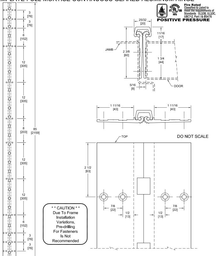
PEMKO Template Full Mortise Continuous Geared Aluminum Hinges CFM85SLF-HD/DFM85SLF-HD are made to conform to this drawing. PEMKO CFM85SLF-HD/DFM85SLF-HD hinges can be supplied with Electric Functions - See Electrical Application Section. Machine Screw Size - No. 12-24 x 7/16 FHUC Thread-forming.
