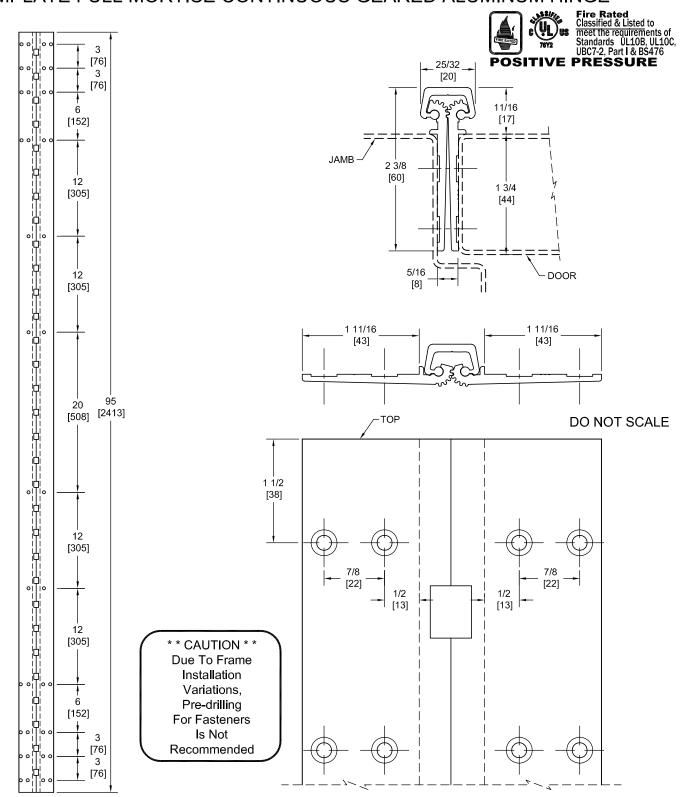
PEMKO Template Full Mortise Continuous Geared Aluminum Hinges CFM95SLF-HD/DFM95SLF-HD are made to conform to this drawing. PEMKO CFM95SLF-HD/DFM95SLF-HD hinges can be supplied with Electric Functions - See Electrical Application Section. Machine Screw Size - No. 12-24 x 7/16 FHUC Thread-forming.
