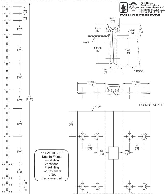
PEMKO Template Full Mortise Continuous Geared Aluminum Hinges CFM83SLI-HD/DFM83SLI-HD are made to conform to this drawing. PEMKO CFM83SLI-HD/DFM83SLI-HD hinges can be supplied with Electric Functions - See Electrical Application Section. Machine Screw Size - No. 12-24 x 7/16 FHUC Thread-forming.
