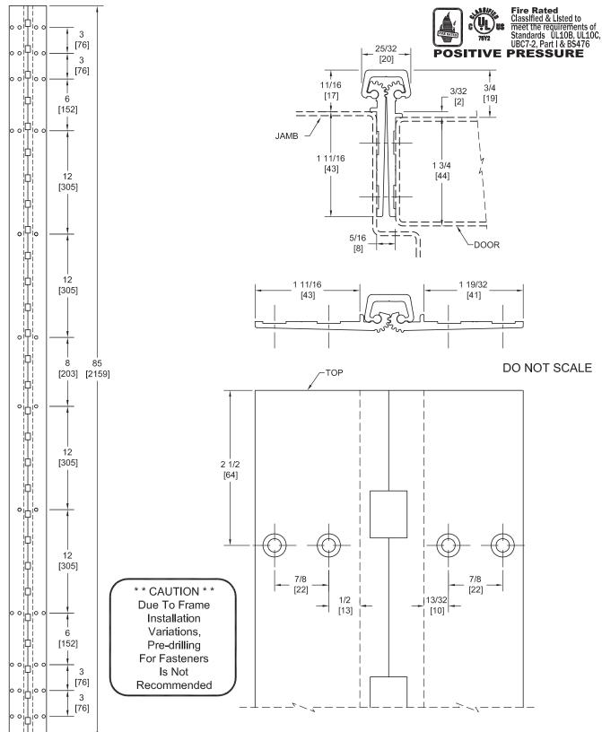
PEMKO Template Full Mortise Continuous Geared Aluminum Hinges CFM85SLI-HD/DFM85SLI-HD are made to conform to this drawing. PEMKO CFM85SLI-HD/DFM85SLI-HD hinges can be supplied with Electric Functions - See Electrical Application Section. Machine Screw Size - No. 12-24 x 7/16 FHUC Thread-forming.
