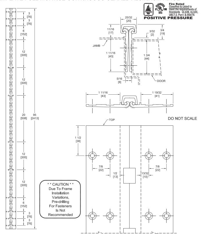
PEMKO Template Full Mortise Continuous Geared Aluminum Hinges CFM95SLI-HD/DFM95SLI-HD are made to conform to this drawing. PEMKO CFM95SLI-HD/DFM95SLI-HD hinges can be supplied with Electric Functions - See Electrical Application Section. Machine Screw Size - No. 12-24 x 7/16 FHUC Thread-forming.
