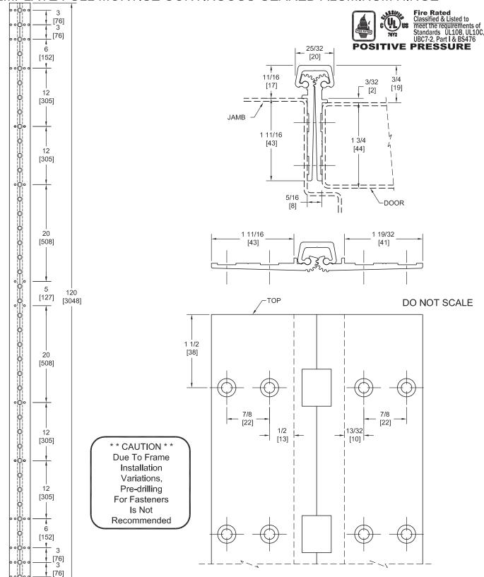
PEMKO Template Full Mortise Continuous Geared Aluminum Hinges CFM120SLI-HD/DFM120SLI-HD are made to conform to this drawing. PEMKO CFM120SLI-HD/DFM120SLI-HD hinges can be supplied with Electric Functions - See Electrical Application Section. Machine Screw Size - No. 12-24 x 7/16 FHUC Thread-forming.
