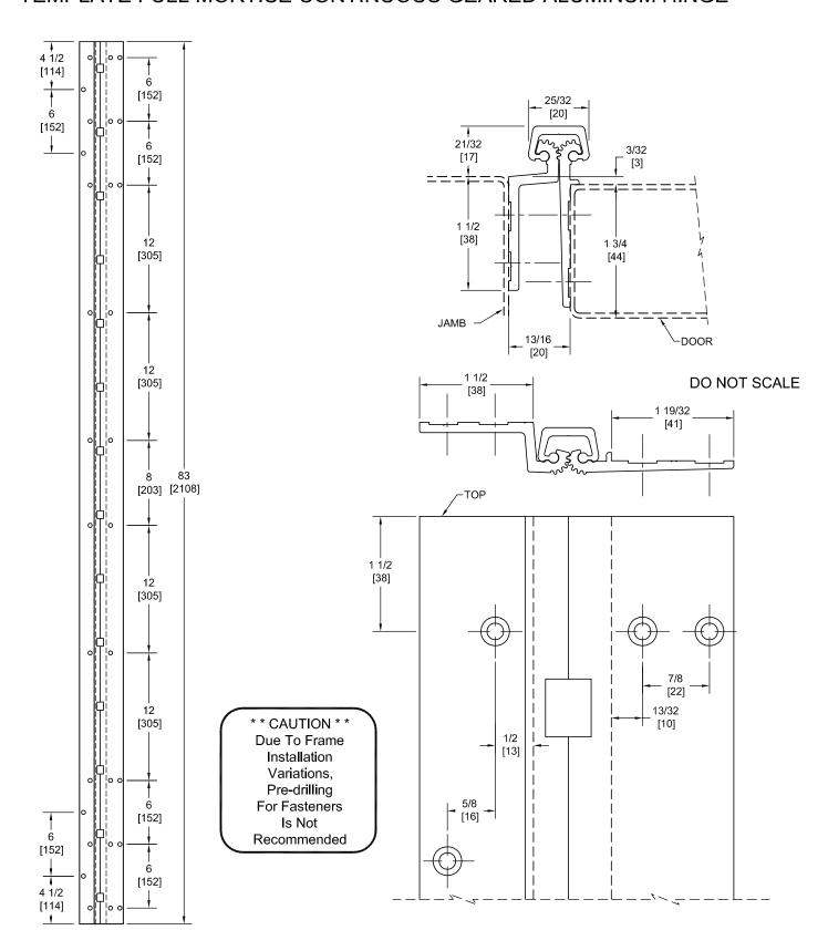
PEMKO Template Full Mortise Continuous Geared Aluminum Hinges CFM83SLISF/DFM83SLISF are made to conform to this drawing. Machine Screw Size - No.  $12-24 \times 7/16$  FHUC Thread-forming.
