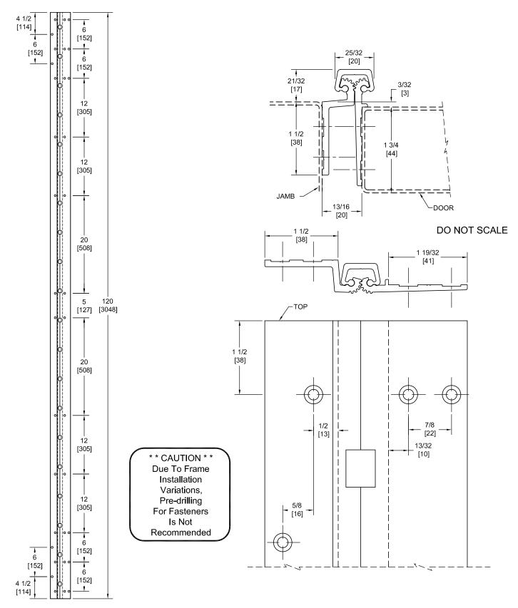
PEMKO Template Full Mortise Continuous Geared Aluminum Hinges CFM120SLISF/DFM120SLISF are made to conform to this drawing. Machine Screw Size - No. 12-24 x 7/16 FHUC Thread-forming.
