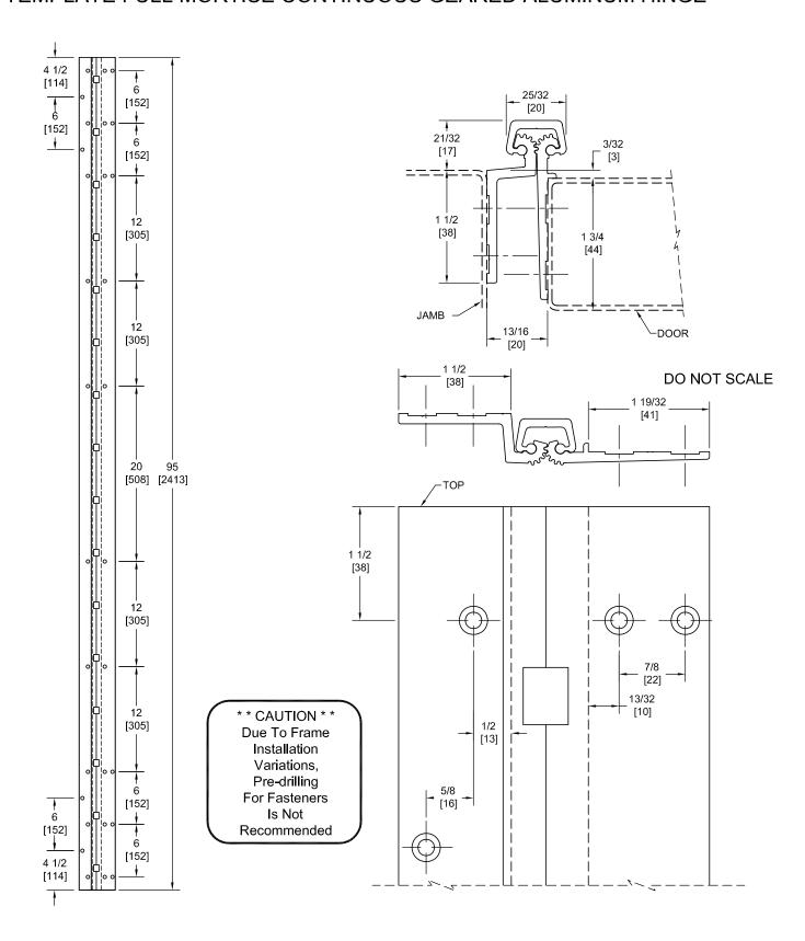
PEMKO Template Full Mortise Continuous Geared Aluminum Hinges CFM95SLISF/DFM95SLISF are made to conform to this drawing. Machine Screw Size - No.  $12-24 \times 7/16$  FHUC Thread-forming.
