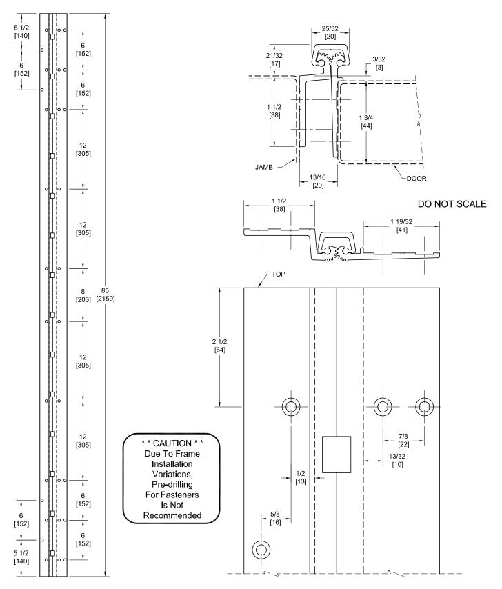
PEMKO Template Full Mortise Continuous Geared Aluminum Hinges CFM85SLISF/DFM85SLISF are made to conform to this drawing. Machine Screw Size - No. 12-24 x 7/16 FHUC Thread-forming.
