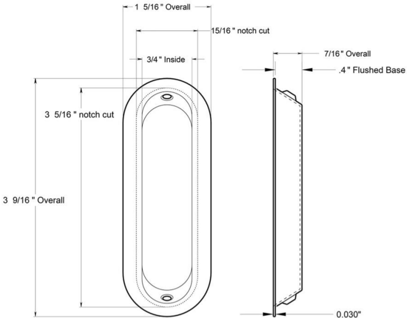
Cut 15/16" x 3-5/16" x 1/2" door notch to fit flush pull base.
