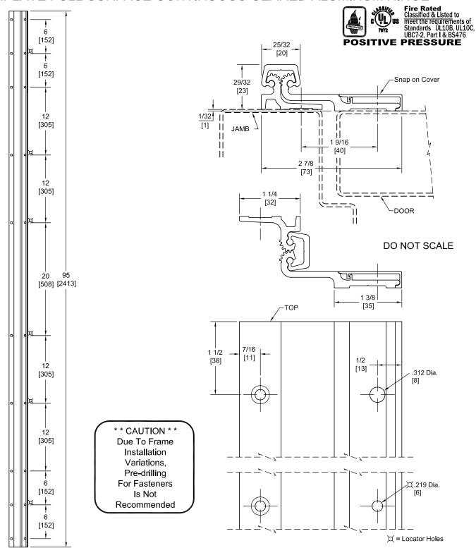
PEMKO Template Full Surface Continuous Geared Aluminum Hinges CFS95/DFS95 are made to conform to this drawing. PEMKO CFS95/DFS95 hinges can be supplied with Electric Functions - See Electrical Application Section.
