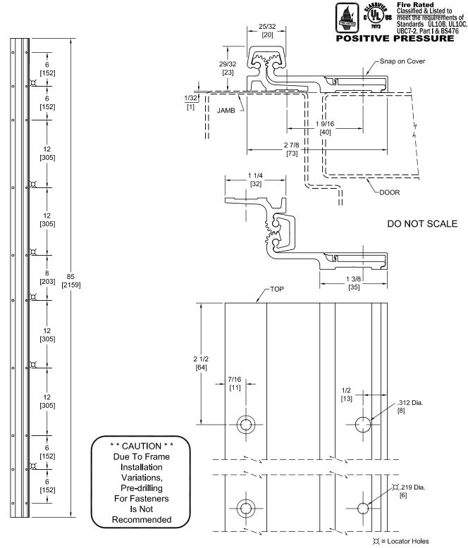
PEMKO Template Full Surface Continuous Geared Aluminum Hinges CFS85/DFS85 are made to conform to this drawing. PEMKO CFS85/DFS85 hinges can be supplied with Electric Functions - See Electrical Application Section.
