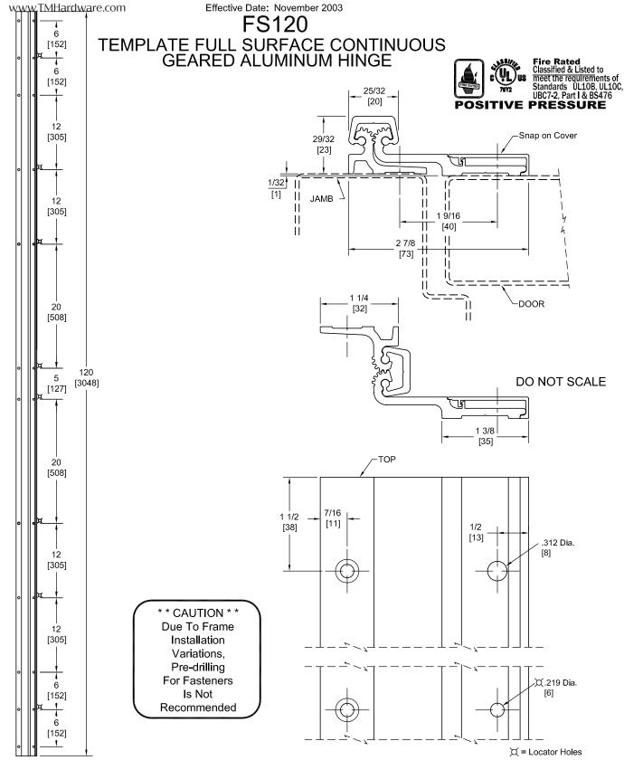
PEMKO Template Full Surface Continuous Geared Aluminum Hinges CFS120/DFS120 are made to conform to this drawing. PEMKO CFS120/DFS120 hinges can be supplied with Electric Functions - See Electrical Application Section.
