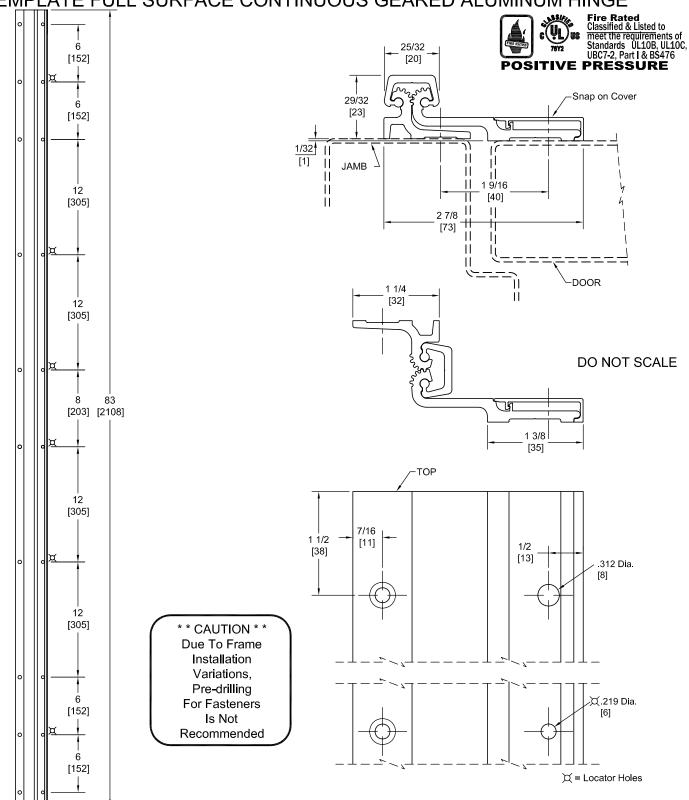
PEMKO Template Full Surface Continuous Geared Aluminum Hinges CFS83/DFS83 are made to conform to this drawing. PEMKO CFS83/DFS83 hinges can be supplied with Electric Functions - See Electrical Application Section.
