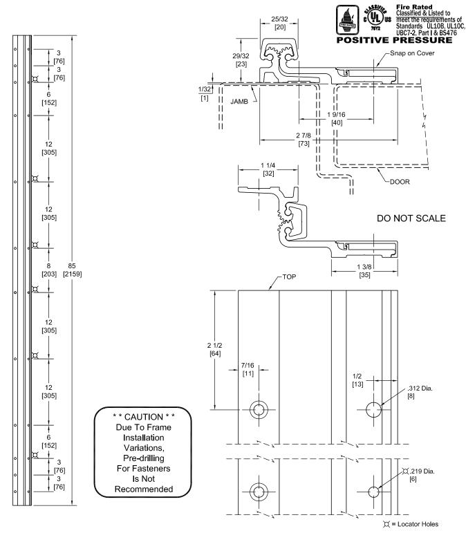
PEMKO Template Full Surface Continuous Geared Aluminum Hinges CFS85HD/DFS85HD are made to conform to this drawing. PEMKO CFS85HD/DFS85HD hinges can be supplied with Electric Functions - See Electrical Application Section.
