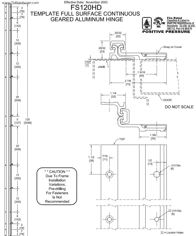
PEMKO Template Full Surface Continuous Geared Aluminum Hinges CFS120HD/DFS120HDare made to conform to this drawing. PEMKO CFS120HD/DFS120HD hinges can be supplied with Electric Functions - See Electrical Application Section. Machine Screw Size - Jamb Leaf - No. 12-24 x 7/16 FHUC Thread-forming.
