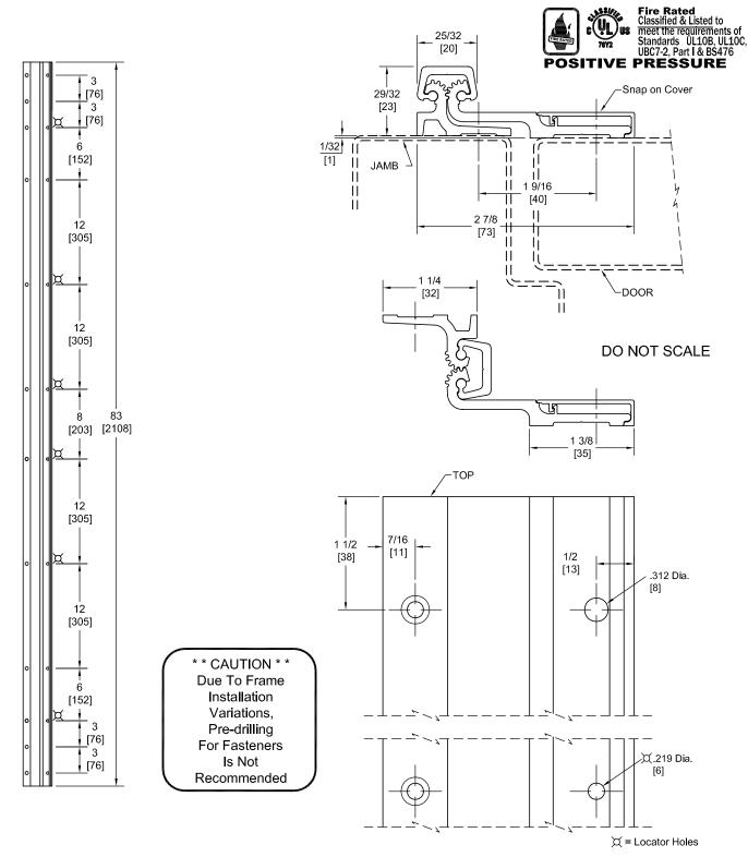
PEMKO Template Full Surface Continuous Geared Aluminum Hinges CFS83HD/DFS83HD are made to conform to this drawing. PEMKO CFS83HD/DFS83HD hinges can be supplied with Electric Functions - See Electrical Application Section. Machine Screw Size - Jamb Leaf - No. 12-24 x 7/16 FHUC Thread-forming.
