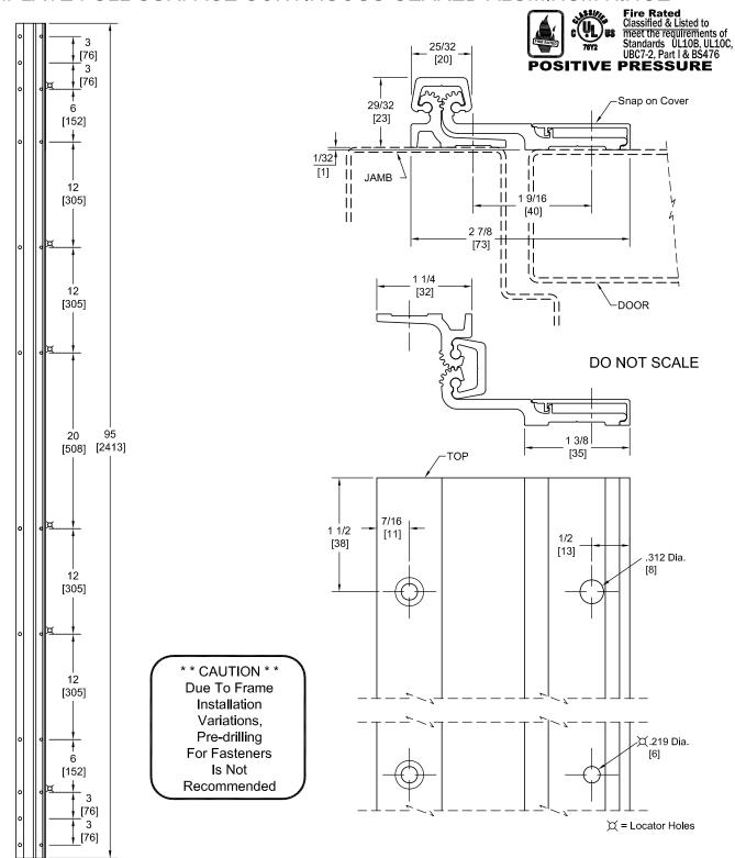
PEMKO Template Full Surface Continuous Geared Aluminum Hinges CFS95HD/DFS95HD are made to conform to this drawing. PEMKO CFS95HD/DFS95HD hinges can be supplied with Electric Functions - See Electrical Application Section. Machine Screw Size - Jamb Leaf - No. 12-24 x 7/16 FHUC Thread-forming.
