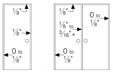
\* Certain door and frame conditions may require an extra 1/32"-1/16" clearance. Excessive clearance on fire rated assemblies may violate the requirements of NFPA 80.
