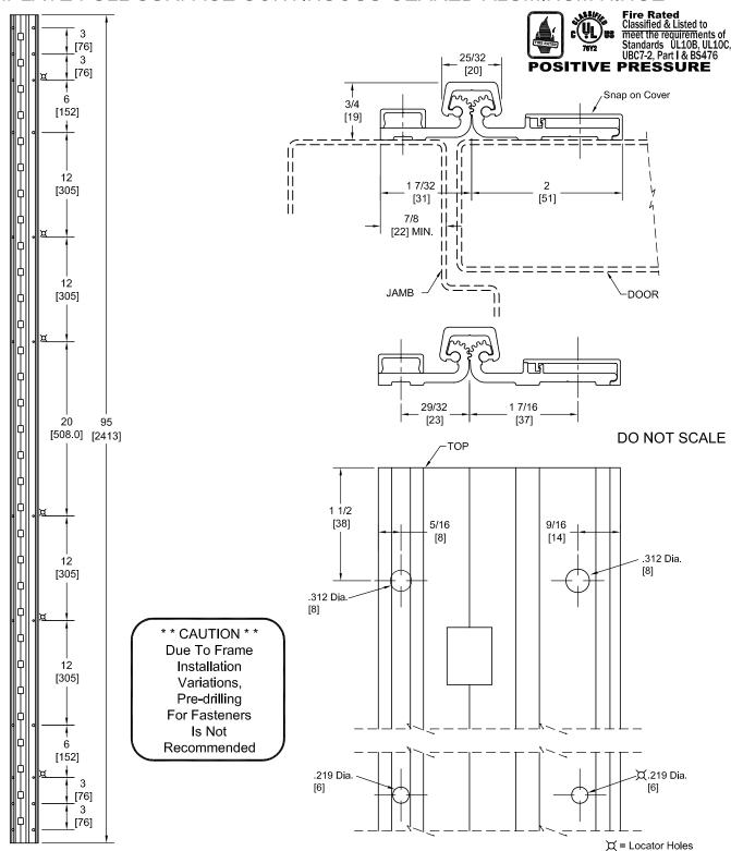
PEMKO Template Full Surface Continuous Geared Aluminum Hinges CFS95CP-HD/DFS95CP-HD are made to conform to this drawing. Machine Screw Size - Jamb Leaf - No. 1/4-20 x 5/8 Self-tapping Security Torx (Tip No. T-27).
