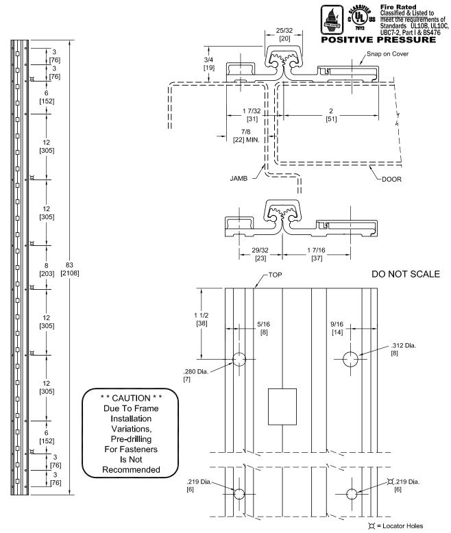
PEMKO Template Full Surface Continuous Geared Aluminum Hinges CFS83CP-HD/DFS83CP-HD are made to conform to this drawing. Machine Screw Size - Jamb Leaf - No. 1/4-20 x 5/8 Self-tapping Security Torx (Tip No. T-27).
