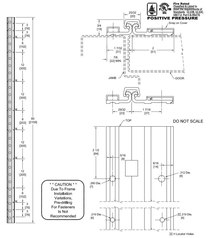
PEMKO Template Full Surface Continuous Geared Aluminum Hinges CFS85CP-HD/DFS85CP-HD are made to conform to this drawing. Machine Screw Size - Jamb Leaf - No. 1/4-20 x 5/8 Self-tapping Security Torx (Tip No. T-27).
