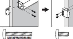
Install Required Support Screws
