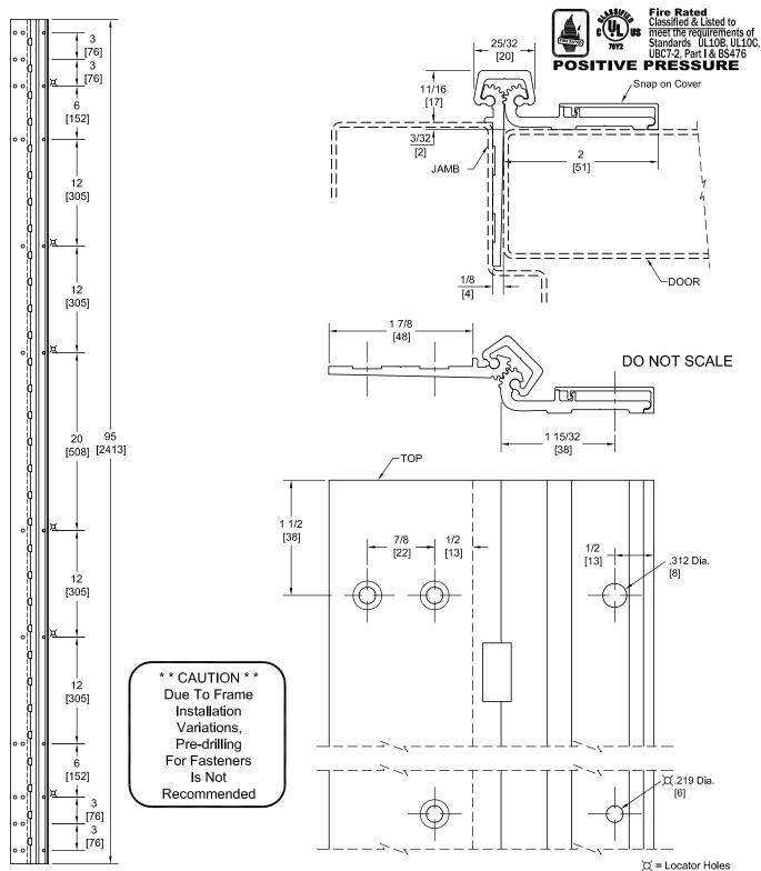
PEMKO Template Full Surface Continuous Geared Aluminum Hinges CHS95HD/DHS95HD are made to conform to this drawing. PEMKO CHS95HD/DHS95HD hinges can be supplied with Electric Functions - See Electrical Application Section.
