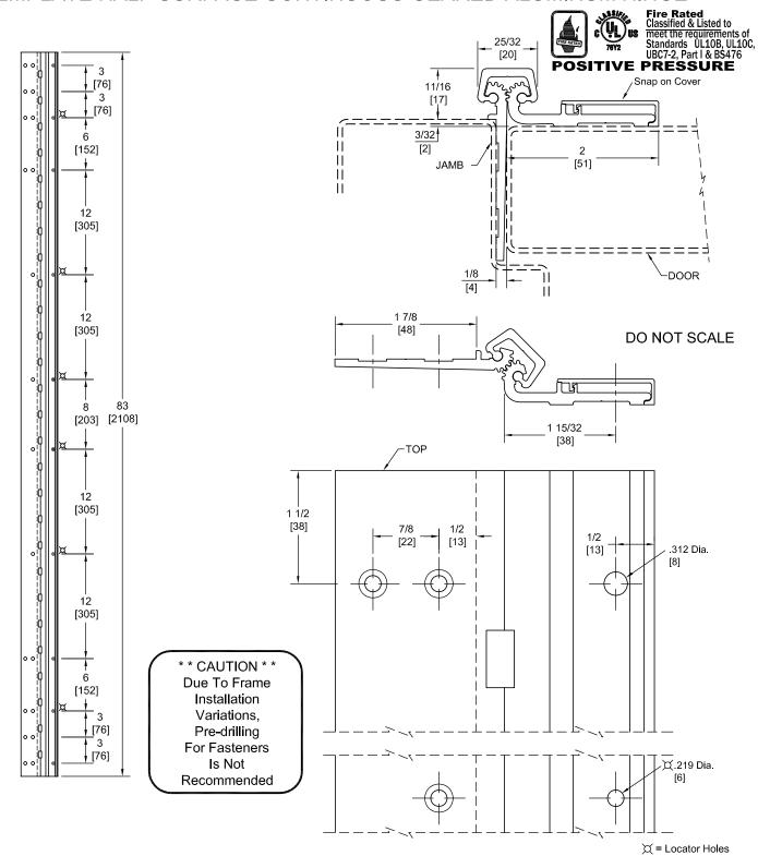
PEMKO Template Full Surface Continuous Geared Aluminum Hinges CHS83HD/DHS83HD are made to conform to this drawing. PEMKO CHS83HD/DHS83HD hinges can be supplied with Electric Functions - See Electrical Application Section.
