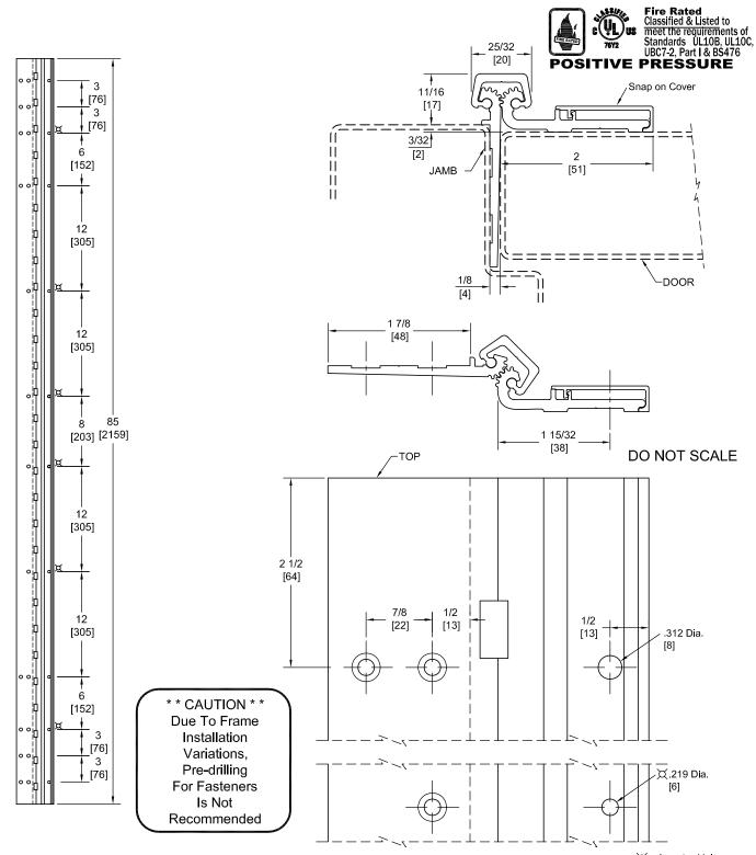
PEMKO Template Full Surface Continuous Geared Aluminum Hinges CHS85HD/DHS85HD are made to conform to this drawing.
