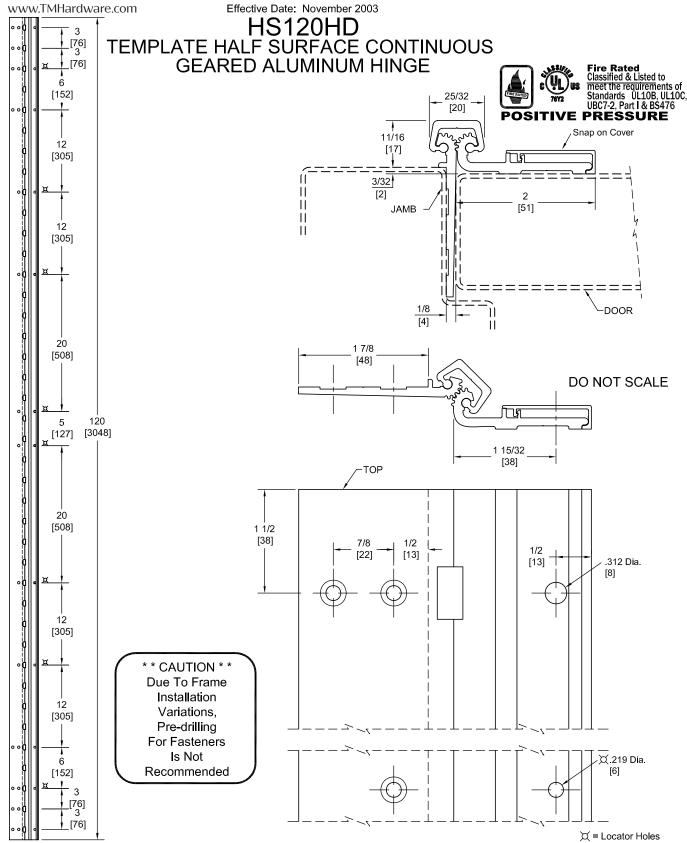
PEMKO Template Full Surface Continuous Geared Aluminum Hinges CHS120HD/DHS120HD are made to conform to this drawing. PEMKO CHS120HD/DHS120HD hinges can be supplied with Electrical Functions - See Electrical Application Section.
