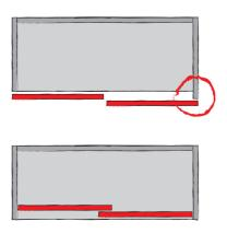
**Overlay sliding doors** conceal – viewed from the front – the carcase side, the top panel and bottom panel. This makes the front panels the dominant design element of a piece of furniture. Please note: for furniture designed with two doors, the two carcase sides must be produced in different depths.
