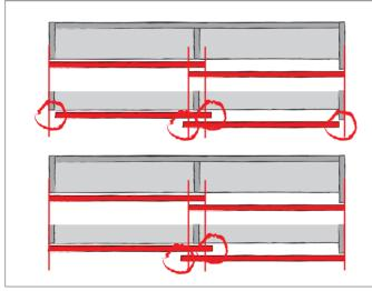
The door reveal is the extent to which the door overlaps the carcase side.
