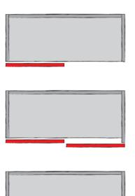
**1-track sliding doors** do not close off furniture completely. The door only conceals individual furniture segments and can be pushed to the side. Typical application: the living room combination in which the TV set disappears behind the sliding door after use.
