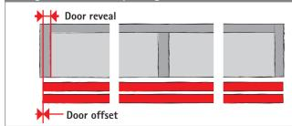
The rear door must produce the same door reveal as the forward door. It must be noted here that this requires the use of special profiles.
