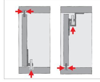
Bottom running sliding doors stand on rollers along their bottom edge and are stabilised by a guide at the top edge of the door. Given the uncomplicated carcase construction, predominantly low door weights and straightforward installation, bottom running doors are seen as the optimum gateway to constructing sliding door cabinets.
