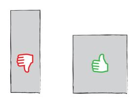
Key to selecting the appropriate system: format and material of the sliding door. In terms of format, bear in mind that wider doors run far more stably than narrow, tall sliding doors. Rule of thumb: the sliding door width should be at least half the height of the door.
