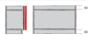
With a simple trick, the fitting technology can be installed largely **out of view on the top panel**: the top panel is lowered by 60 mm. Proviso: the piece of furniture is a tall cabinet with a top panel that is positioned out of sight.
