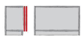
On low cabinets, the top panel is always visible. In this case, carcase and top panel are conventionally mounted at right angles and the fitting technology is either attached **in front of or in the top or bottom panel**. The doors close flush at the top – a neat looking solution. Incidentally: the cabinet here is designed in the same way as hinged door cabinets. Benefit: subsequent conversion from hinged door to sliding door system can be done with little effort.
