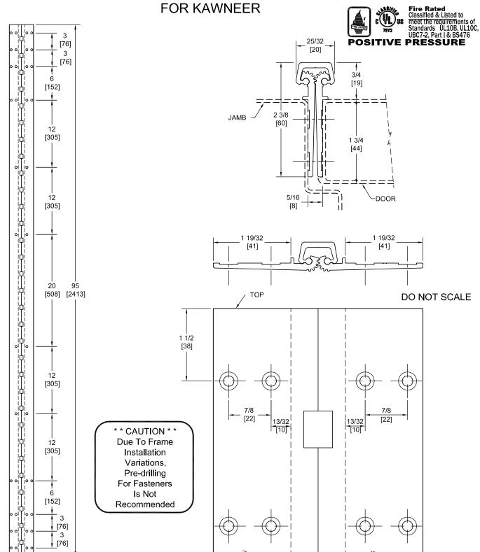
PEMKO Template Full Mortise Continuous Geared Aluminum Hinges KCFM95HD/KDFM95HD are made to conform to this drawing. PEMKO KCFM95HD/KDFM95HD hinges can be supplied with Electric Functions - See Electrical Application Section. Machine Screw Size - No. 12-24 x 7/16 FHUC Thread-forming.
