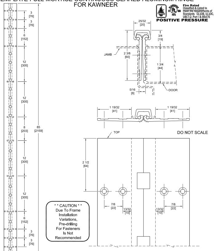
PEMKO Template Full Mortise Continuous Geared Aluminum Hinges KCFM85HD/KDFM85HD are made to conform to this drawing. PEMKO KCFM85HD/KDFM85HD hinges can be supplied with Electric Functions - See Electrical Application Section. Machine Screw Size - No. 12-24 x 7/16 FHUC Thread-forming.
