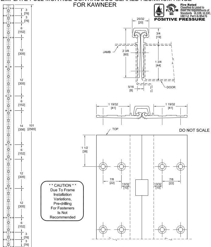
PEMKO Template Full Mortise Continuous Geared Aluminum Hinges KCFM101HD/KDFM101HD are made to conform to this drawing. PEMKO KCFM101HD/KDFM101HD hinges can be supplied with Electric Functions - See Electrical Application Section. Machine Screw Size - No. 12-24 x 7/16 FHUC Thread-forming.
