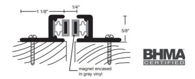
Maximum distance between two pieces 5/16". Install only on outside of out-swinging doors or inside of in-swinging doors.
