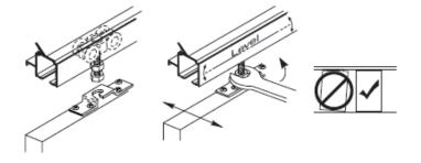
8. Position and secure retaining stop.
