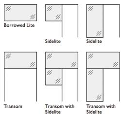
The maximum visible glass area allowed for side lites, borrowed lites, and glass transoms is 4,704 square inches with a maximum length of 106" in any one direction.
