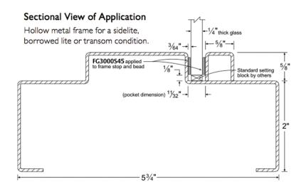
Technical Data For 20- And 45-Minute Hollow Metal Screens Equipped With FG3000S45 (Sidelite/Borrowed Lite/Transom Lite Applications)
