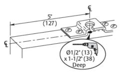
3. Insert hangers and retaining stop.
