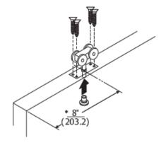
\*From door edge to centerline of hanger bolt and plate.
