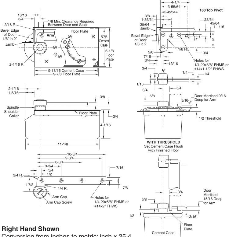
Conversion from inches to metric: inch x 25.4 Rixson designed threshold available on request.
