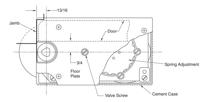
Closing speed can be adjusted to suit local conditions and requirements. With a screw driver turn the adjustment screw that projects through the floor plate or threshold, either in or out as the case may be until the desired action is attained. Turn this valve screw to the right, clockwise, to decrease
