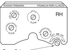
Do not use Backcheck as deadstop. This is an intensity valve not speed control.
