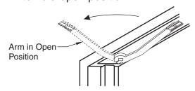
b. Remove arm from spindle.
